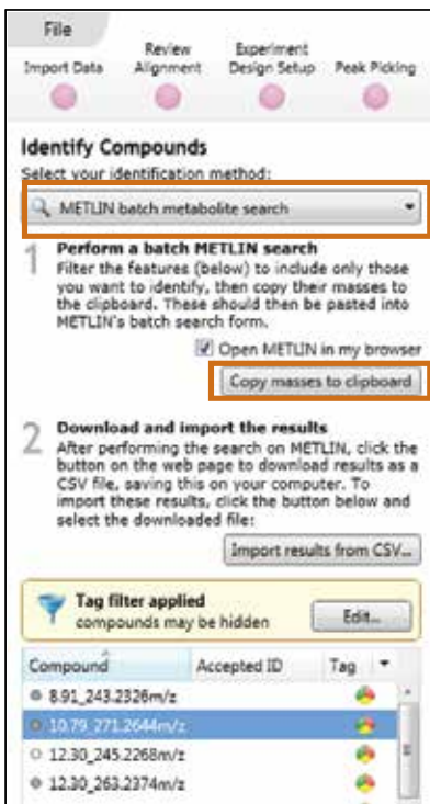
Figure 10. Screen capture of the compound identification page in Progenesis QI. Highlighted areas show the ease of batch submission for markers of interest to an external (METLIN) database.
